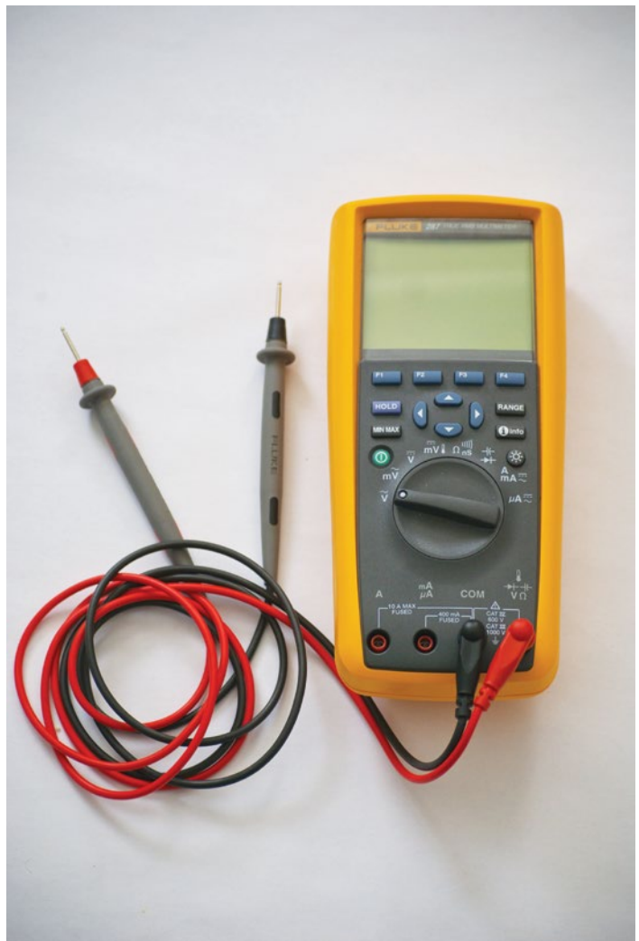
A high-impedance multimeter, excellent for digital troubleshooting
