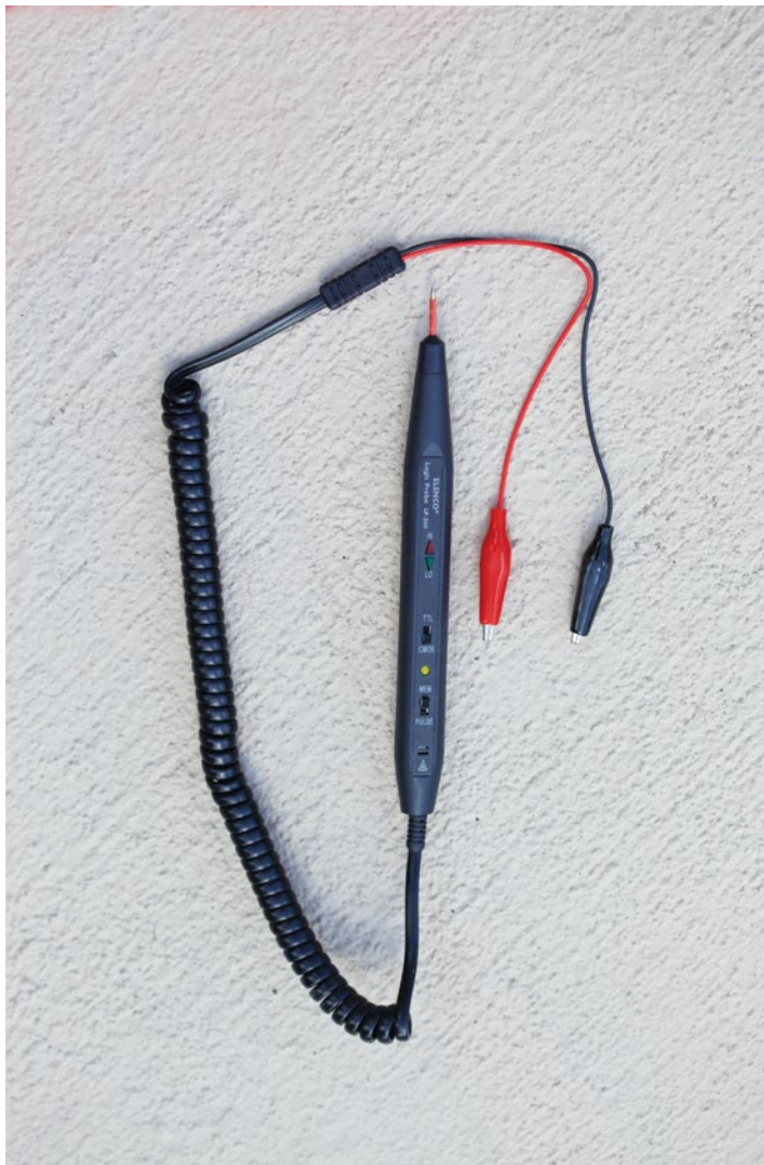
A digital logic probe is a digital troubleshooter's basic instrument.
