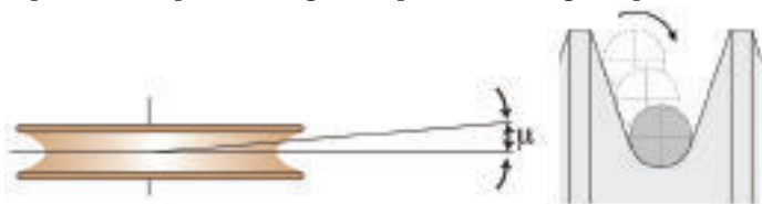
Monitor your fleet angles (the angle of a rope as it leaves one sheave and connects with another), as too wide an angle can result in premature wear of the rope. A 4% fleet angle will reduce rope life by 30%.
