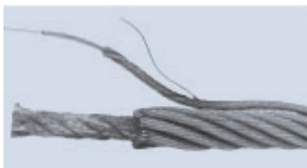
Figure 1: Fiber core, strand and wire
