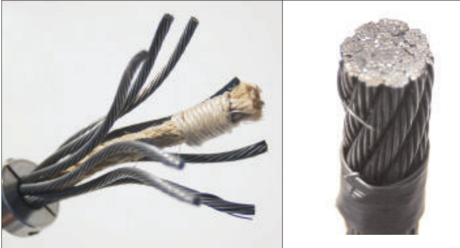
8 X 19 Right regular lay sisal-core rope
