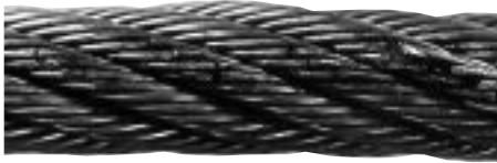
Figure 32: Inner wire breaks are visible when stretched.
