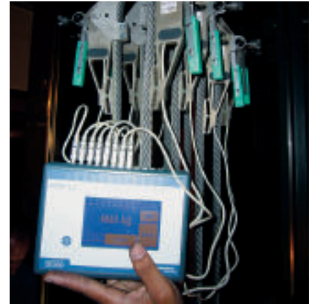
Figure 26: Rope Tensile Force measurement
