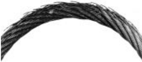
Figure 33: Inner wire breaks are visible when bent.
