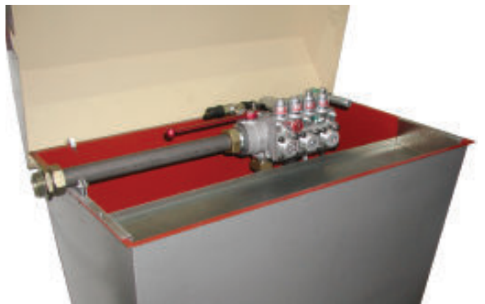
Figure 3: A hydraulic power-unit tank with lid to conceal the control valve
