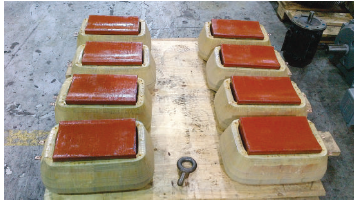
(l-r) Gearless field coils before refurbishment and after, installed on shoe coils
