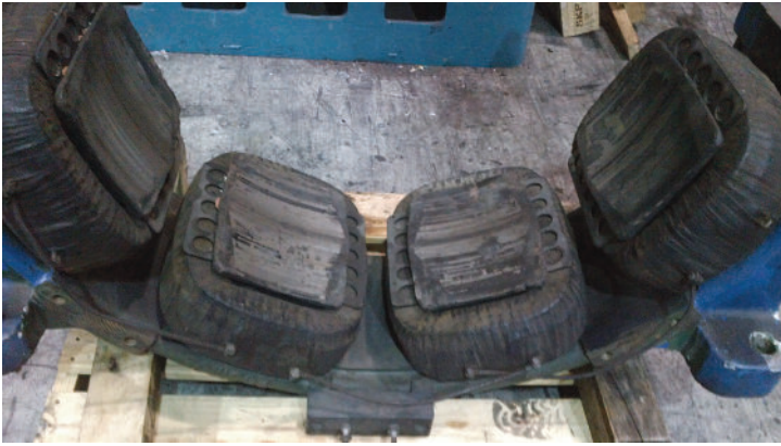
(l-r) Gearless field coils before refurbishment and after, installed on shoe coils
