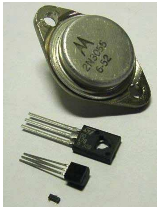
Figure 1: Transistor packages in order from top to bottom: TO-3, TO-126, TO-92 and SOT-23 (photo by Transisto)
