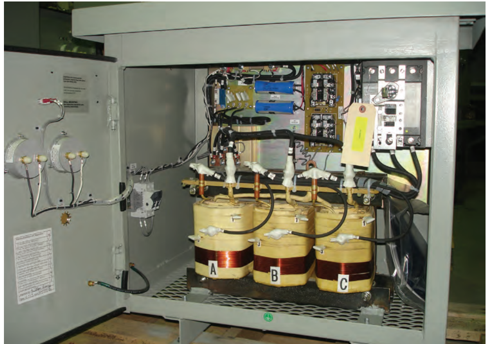
This Kinetics Industries 20-kW single-elevator rectifier with 208-V, three-phase input includes an AC-input circuit breaker with through-the-door operator for safety lockout/tagout, a diode full-wave bridge rectifier and a 20%-of-rectifier regenerative-absorption circuit.
