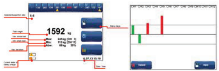
Figure 4: (l-r) Seen here are a control unit for a mobile system in which sensors connect by USB to each rope (or belt sensor) and a unit using tensioning function with an example of a five-rope elevator where one rope is set as a reference for the remaining four. If rope CH5 is loosened or CH2 is tightened, the other ropes relatively change.
