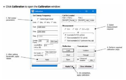
Setting VNA field calibration parameters
