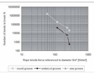
Figure 6: Number for bends to break in various groove types for  $\ensuremath{8x19S\text{-NFC}}$  rope
