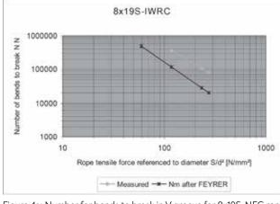
Figure 4a: Number for bends to break in V groove for 8x19S-NFC rope
