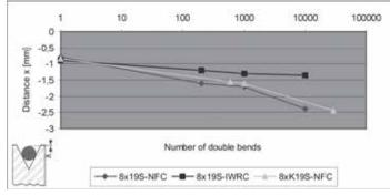
Figure 11: Descent into the V groove at 11.7kN rope tension
