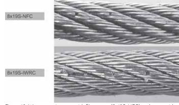
Figure 10: Wear zones in ropes with fiber cores (8x19S-NFC) and ropes with steel core (8x19S-IWRC)
