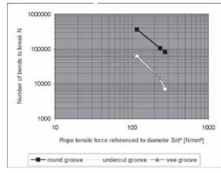
Figure 7: Number for bends to break in various groove types for  $8 \times 19 \mbox{S-NFC}$  rope
