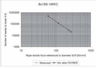
Figure 3b: Number for bends to break in round groove for 8x19S-IWRC rope
