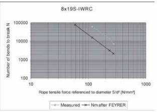
Figure 5b: Number for bends to break in undercut groove for 8x19S-IWRC rope
