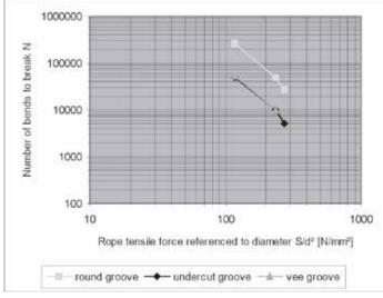
Figure 8: Number for bends to break in various groove types for 8xK19S-NFC rope
