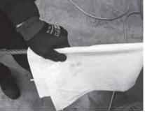
Method for checking for lubrication
