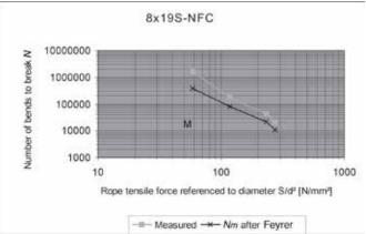
Figure 3a: Number for bends to break in round groove for 8x19S-NFC rope
