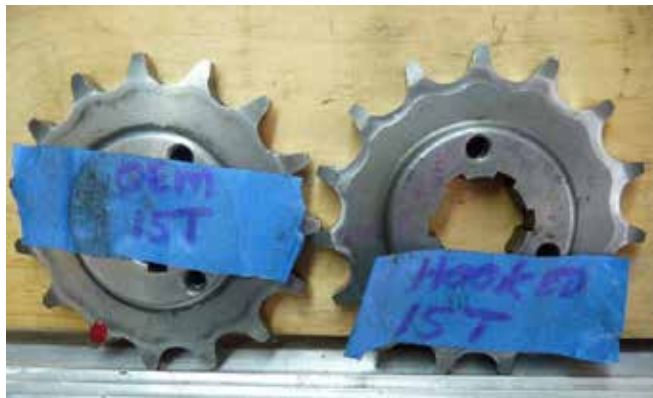
New (left) and "hooked tooth" (right) sprockets
